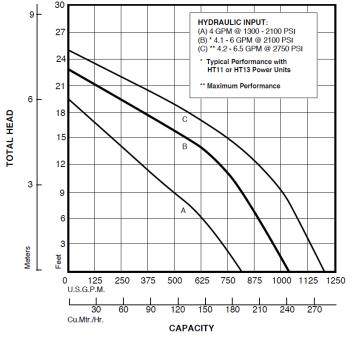
Curves are based on pumping water at 60°F. For performance curves other than shown above, consult factory.
